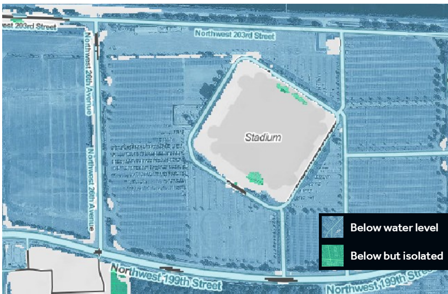
Hard Rock Stadium, Miami Gardens, Fla., showing areas below a water level of 6 feet above the local high tide line, which could occur through combinations of sea level rise, tide, and storm surge.
